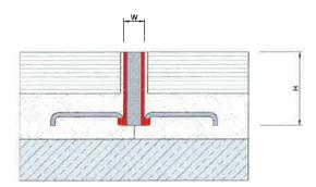
Can be manufactured in stainless steel, brass or aluminium depending on the anticipated chemical, mechanical, electro-chemical or any other load to which the floor could be exposed. Recommended for mortal-laid floors. Ideal for heavy pedestrian or vehicle traffic.
