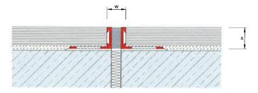
Profiles at 2, 3 and 4.5 mm heights are applied at epoxy, linoleum, PVC coated floors. Prevents the cracking of epoxy coating and gives a decorative aspect. Economize at labour cost and save time during epoxy application.
